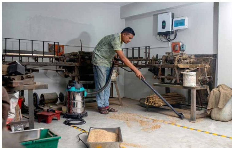
Collecting metal dust using industrial vacuums reduces workshop pollution and helps turning waste into extra revenue.
