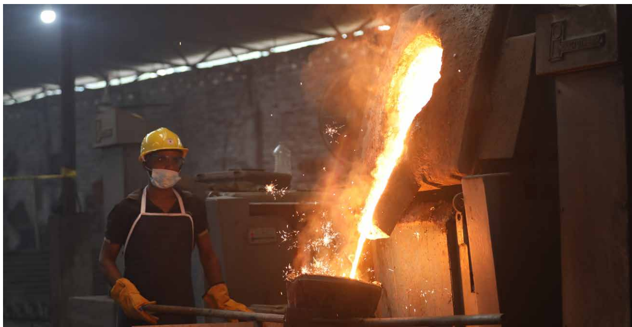
The coal-fired cupola furnace has been replaced by an electric induction furnace that has eliminated GHG emissions and ash.
