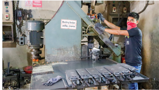
Shoe soles being made out of recycled waste generated from the footwear factories around the cluster
